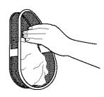
**STEP 4.** Put the lint screen and cover back together and push firmly back into place.
